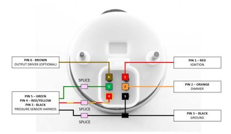
**PIN 1 – Red:** <u>Ignition</u>; Connect to one wire of the included fuse holder using the included crimp splice, and the other wire of the fuse holder connected to a circuit that switches on with the key switch. Install the included 1-amp fuse in the fuse holder.
