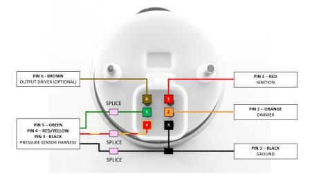
PIN 1 - Red: Ignition; Connect to one wire of the included fuse holder using the included crimp splice, and the other wire of the fuse holder connected to a circuit that switches on with the key switch. Install the included 1-amp fuse in the fuse holder.
