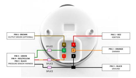
PIN 1 - Red: Ignition; Connect to one wire of the included fuse holder using the included crimp splice, and the other wire of the fuse holder connected to a circuit that switches on with the key switch. Install the included 1-amp fuse in the fuse holder.
