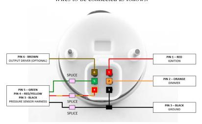
**PIN 1 - Red:** <u>Ignition</u>; Connect to one wire of the included fuse holder using the included crimp splice, and the other wire of the fuse holder connected to a circuit that switches on with the key switch. Install the included 1 amp fuse in the fuse holder.
